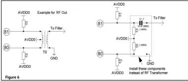
The diagram shows changes in the electrical schematic to reduce the minimum operating frequency of the output signal (see **Figure 6**):
