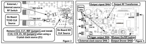
The level of the external clock signal must be within the range of -10 dBm to +10 dBm for a sinusoidal signal. For example, if the signal level from an external generator is +16 dBm, it is necessary to connect it only through an attenuator of at least 6 dBm (16 - 6 = 10). For signals of other waveforms, such as a clipped sine or square wave, the level must be **0.2 - 1 Vpp**.
